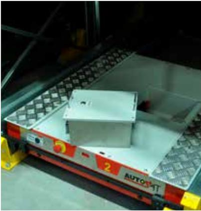
Longlife lithium battery removed for recharging
